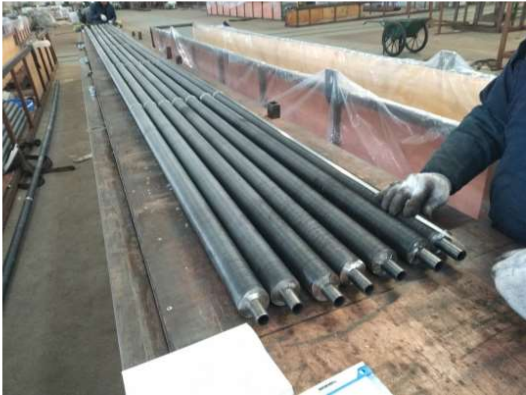
ASTM A179 Fin tubes
